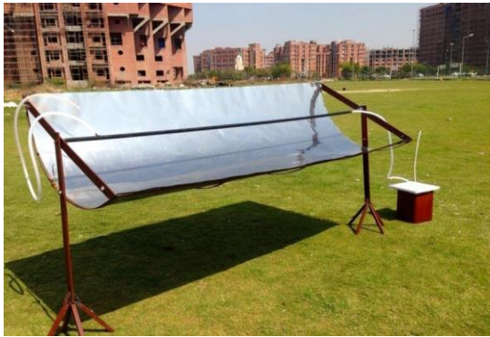
Fig 2b: Working Set up of Solar Thermal Syphon Pump at Sharda Univ Greater Noida campus
